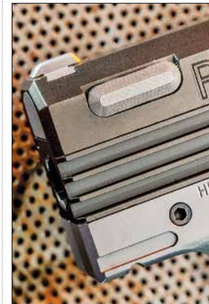
Turning the lever on the left side of the slide, near the muzzle, allows you to remove the recoil spring assembly during the takedown process.
